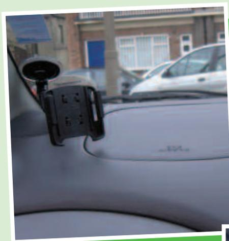
Objects such as this mobile phone bracket, placed in the deployment area for the passenger airbag. This could render the airbag useless in the event of an accident.
