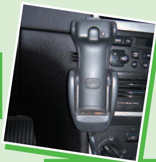
Mobile phone brackets, fire extinguishers, etc, intruding into the examiner's space. They could injure the examiner in the event of an accident.
