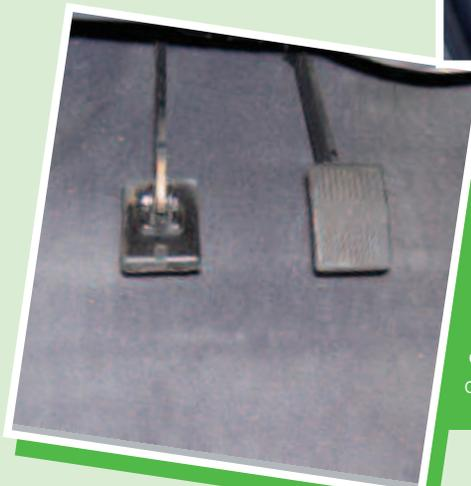
Dual controls incorrectly fitted or adjusted, which could stop them from working when required, or pedals without rubbers which could injure examiners' ankles or legs in a crash.
